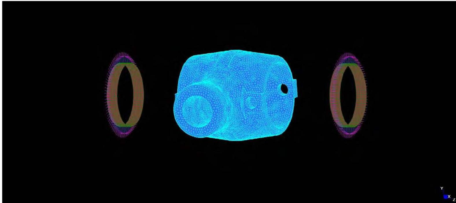
**Bearing race and torque tube as one element. Beam elements representing ball bearings. End of beams constrained in R & Z of the horn cylindrical coordinate system. Bearing is free to rotate in Theta. Global Y constraint at the end of the Counterbalance tube, representing the control cables.**
